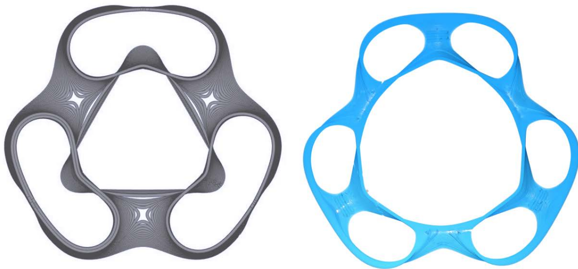
Figure 9. Pinch effect. Layer comparison. (Left) Top view. Section of the object, showing the problem Before around the saddle points, during the simulation with the actual 3mm diameter nozzle and with 1.5mm layer height (Right). Showing the result After applying the mentioned additional forces and the layer modification.
